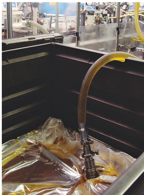
A heavy-duty liner bag inside a bulk tote is filled with up to 330 gal of shampoo for a hotel amenity application such as those in the ProTerra product line, top photo.
