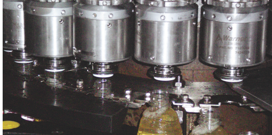
Bottles enter the capper, left, through a feed screw. The magnetic-capping headsets, right, utilize a third magnet that eliminates pulsation, resists rotation and provides smooth capping torque.
