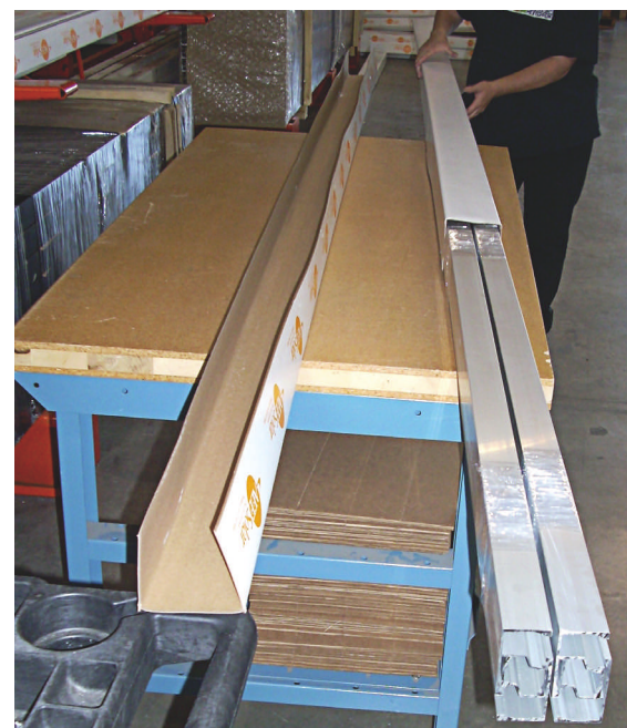
Rails are shrink-wrapped in sets before being set in the laminated paperboard crates.
