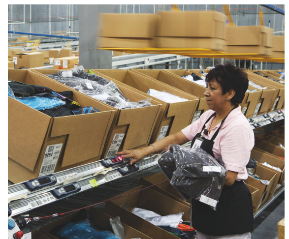
Most products need to be repackaged for shipment to stores, so the put-to-light system assists with store allocations.
