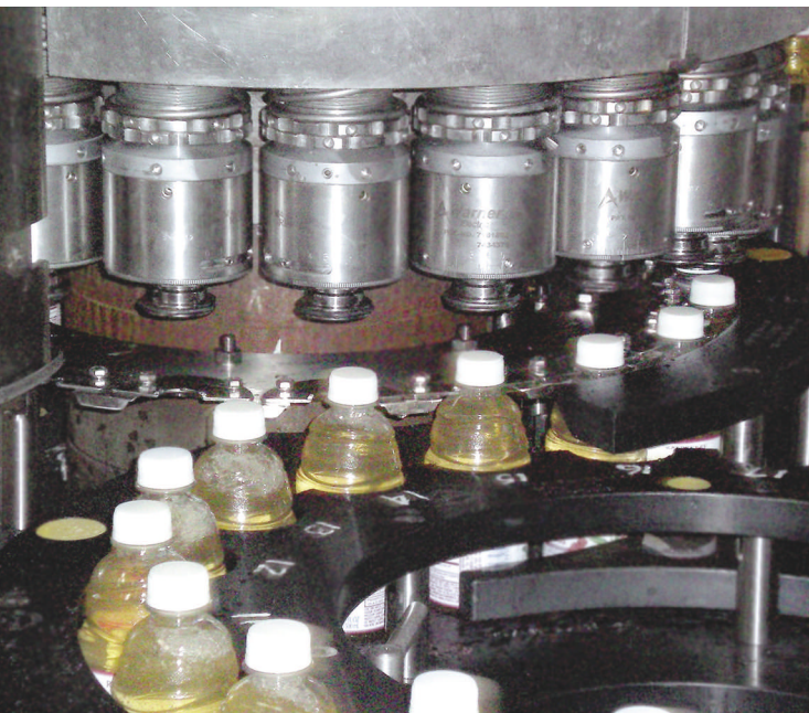
One of the primary advantages of the smooth-torque headsets is that they eliminate cap overtightening.
