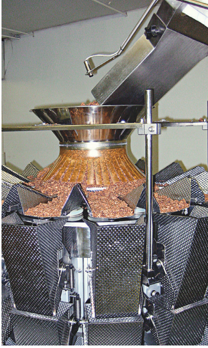
Vibrating dispersion pans transfer the product from a central funnel to 14 radial feeder hoppers, which, in turn, move the product by vibration to the weigh buckets.
