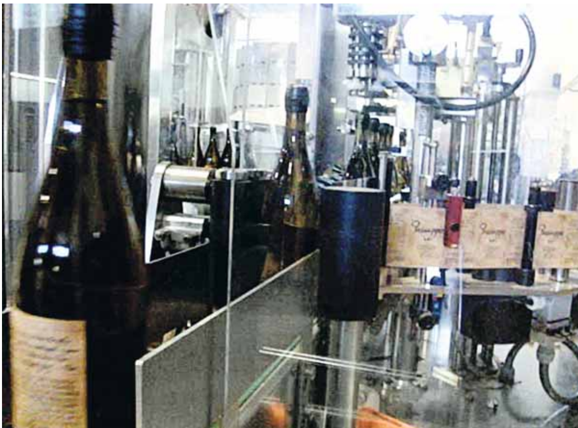
Wine closures are hand-placed but are pressed onto glass bottles by a combination labeler and capsuler machine. After the caps are secured, the bottles travel to a labeling area. Roll-fed labels are then applied.
