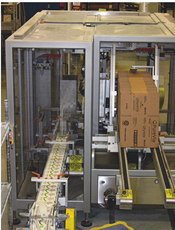
The seven-axes, servo-driven casepacker can pick and erect 20 cases/min. The balcony design provides convenient, full walk-in access to all of the components.
