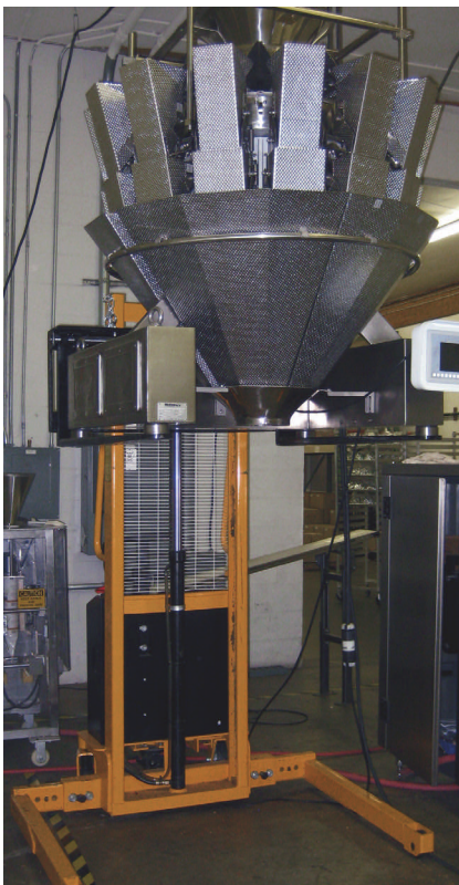
The scale is uniquely installed on a hydraulic jack that is mounted on wheels so it can easily be moved from one bagging machine to the other.
